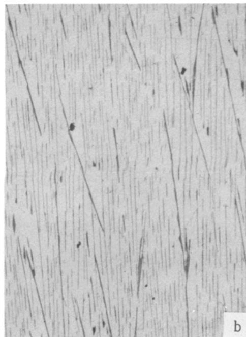
Figure 1 Composite specimen grown at 1 \text{ cm h}^{-1} , exhibiting blade-like fibre morphology. (a) Transverse section, \times 230 ; (b) Longitudinal section, \times 100 .
